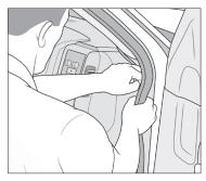
**8.** Tuck cable behind weather stripping, and push stripping in to secure it.
