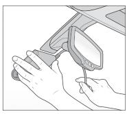
**5.** Remove backing, then press evenly to ensure unit is flush against the glass. Hold to window for 30 seconds.
