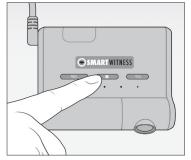
**10.** Hold center button on AP1 camera unit for 5 seconds. Release button, and wait 3 seconds for blinking orange light.
