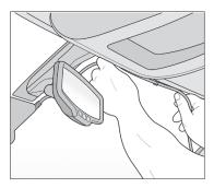
**7.** Remove adhesive backing on clips, and adhere cable to windshield.
