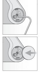
**17.** Tighten the camera angle lock screw, and attach the cover.
