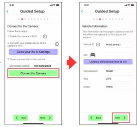
15. Return to the Tool and tap Connect to Camera. You should see the message, "Download request was successful." Next, follow each page's prompts to enter and save calibration information. Pay close attention to vehicle measurement and "Horizon" and "Hood" line settings, as accurate values are crucial to proper device function.
